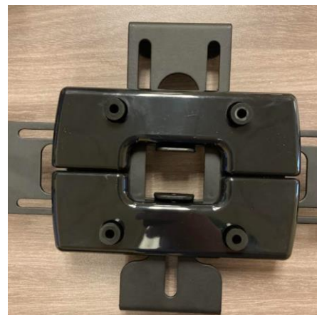
Figure 15. Plastic Covers attached to Clamp
